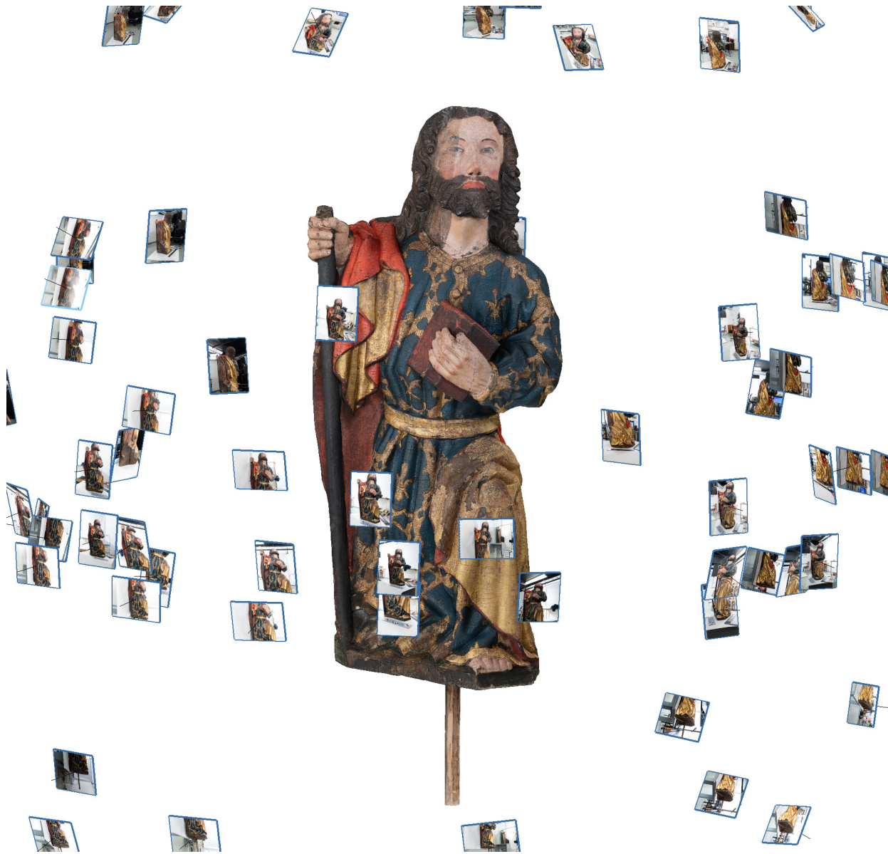
Figure 6. Photogrammetric 3D model of the figure of Philip the Apostle after conservation. (Photos and model: Andres Uueni.)
